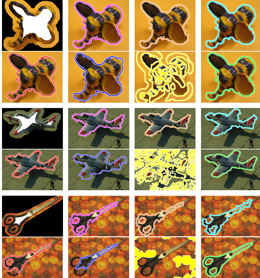
Fig. 5. Example segmentations on the GrabCut dataset images under different magnitudes of noise. For each image, top row: image with seeds, segmentations yielded by graph cuts, random walker, and Meyer flooding, bottom row: segmentations produced by power watershed, DRLSE, RSF and viscous watershed. From top to bottom, the ceramic elephant image is the original one without noise corruption, the fighter jet image is corrupted by a Gaussian noise with \sigma = 0.1 , and the scissors image is corrupted by a Gaussian noise with \sigma = 0.3 .
