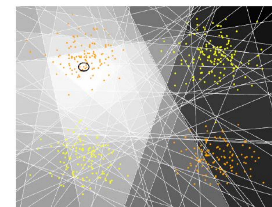
Figure 4. The effect of a single noisy XOR update (circled) on the decision boundaries of a halfspace gated GLN. Sampled hyperplanes for each gate are shown in white.
